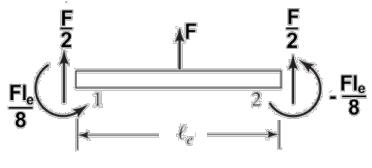
$$v(\xi) = H_1 q_1 + \frac{l_e}{2} H_2 q_2 + H_3 q_3 + \frac{l_e}{2} H_4 q_4$$
