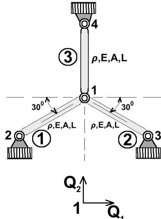
$$E = 200 \text{ GPa}, A = 5,38 \cdot 10^3 \text{ mm}^2, \rho = 7844 \frac{\text{kg}}{\text{m}^3}, L = 3 \text{ m}$$
